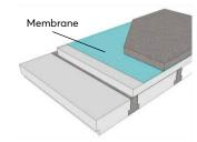
Laying the membrane directly above the beams but beneath the insulation overlay sheet may be suitable where services are pinned onto the insulation overlay sheet. This avoids the possibility of puncturing the membrane with pipe-securing pins.
