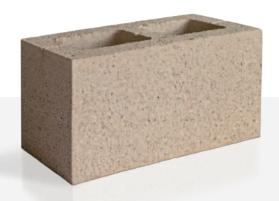
This block is manufactured with full height voids which reduce the unit's overall weight. Steel reinforcement can be located in the block voids which is then surrounded with suitable poured concrete to created reinforced structures.
